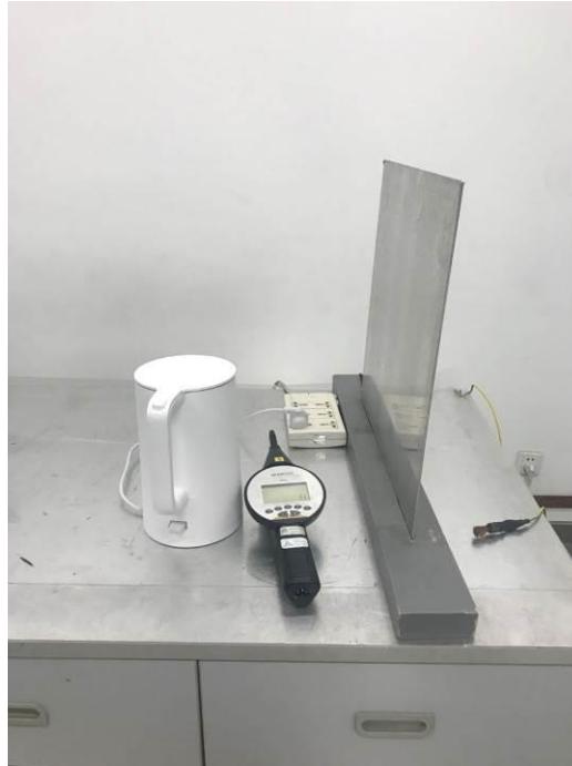
Photograph 4: Set-up for immunity test of fast transient/burst
