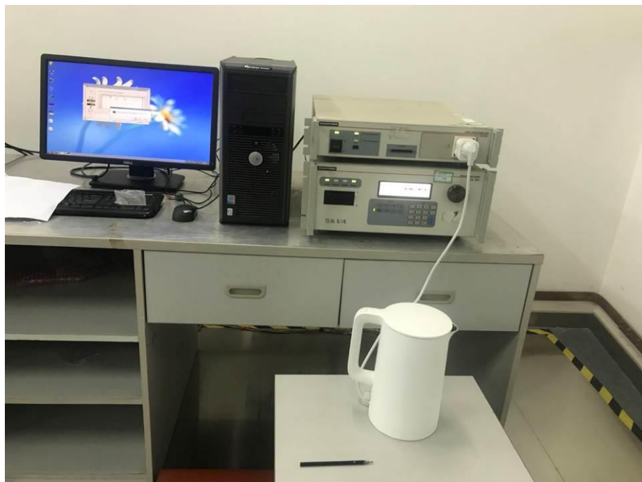
Photograph 8: Set-up for immunity test of harmonic currents and voltage fluctuations and flicker
