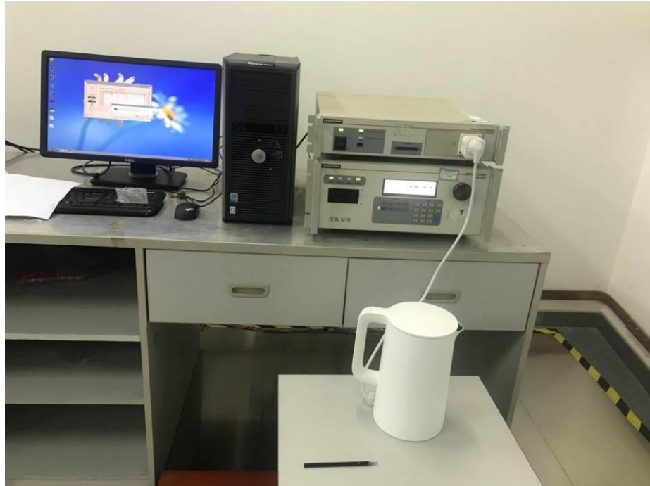
Photograph 8: Set-up for immunity test of harmonic currents and voltage fluctuations and flicker
