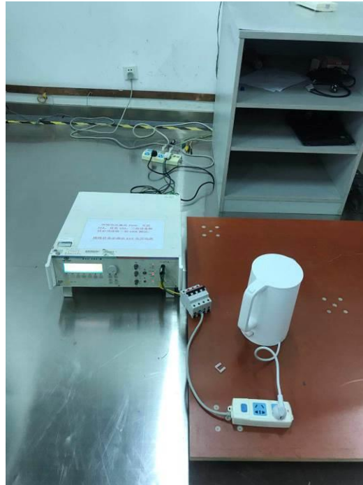
Photograph 5: Set-up for immunity test of surge
