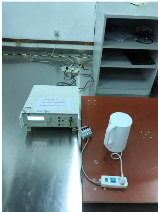
Photograph 4: Set-up for immunity test of fast transient/burst
