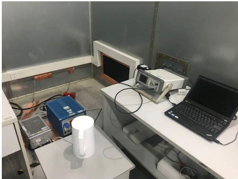
Photograph 2: Set-up for Radiated emission
